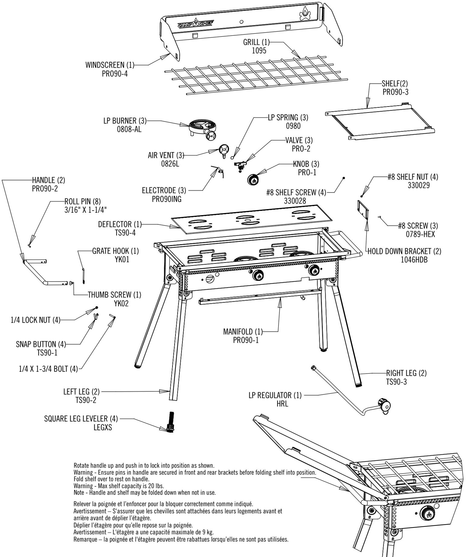
Rotate handle up and push in to lock into position as shown.
