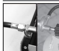
Attach regulator to tank. Check all connections to ensure tightness. With all valves in the off position, apply a soapy water solution to all fittings, valves and connections. Turn gas on at the tank and check for leaks at all connections. Small bubbles will appear if connection leaks. Tighten as needed.
