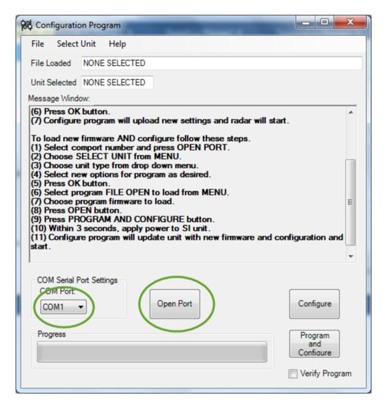
(4) Press the "Configure" button and then power up the G3 unit. (within 5 seconds)
