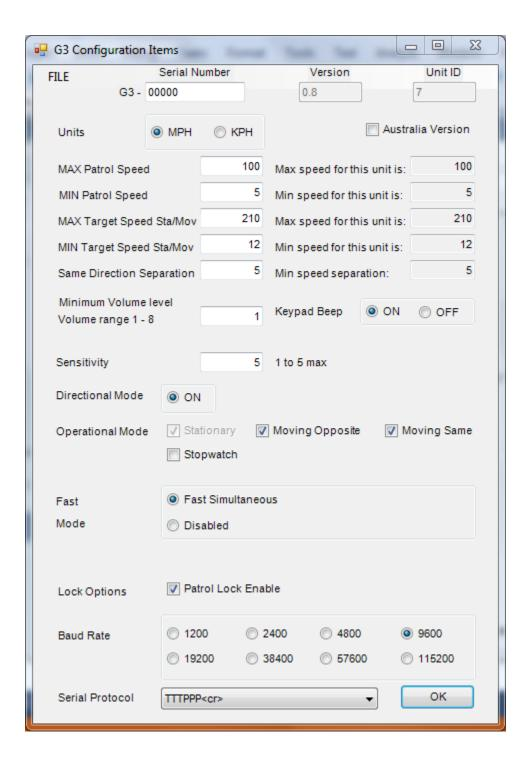
(6) Make selections as desired then click on the OK button in the lower right hand corner to complete the loading of the new selections. You can also load in a predefined configure file using the "FILE" + "OPEN" commands.
