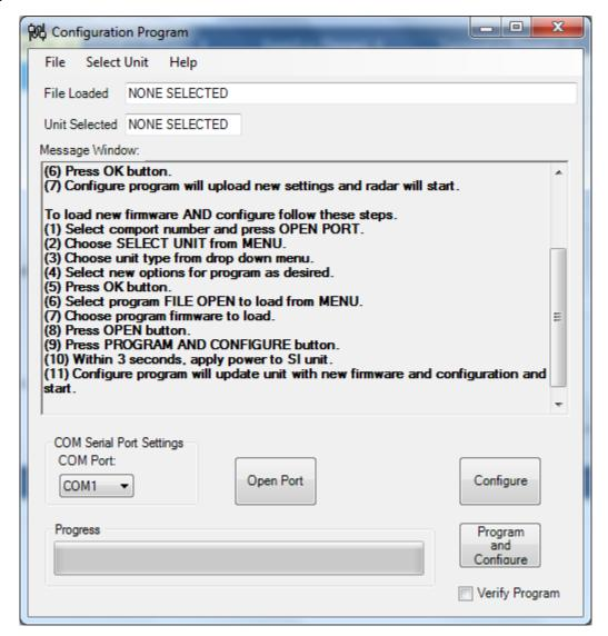
(2) Make sure the COM PORT is set correctly to the proper open port available on your computer.
