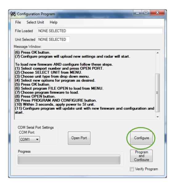
(5) After a 1-5 second delay, the following configuration box will show. (NOTE: the settings in your G3 unit may be different than what is shown here)
