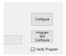
To verify that the flash memory chip on the G3 has programed correctly, you can check the "Verify" box on the main program window. After loading new firmware into the G3, the configure program will test and verify the contents of the flash memory chip to confirm that the code loaded into the G3 matched the firmware that was loaded in.
