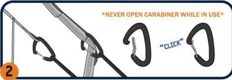
Attach carabiners to straps making sure each carabiner clicks closed and visually check that the gates are closed before use.
