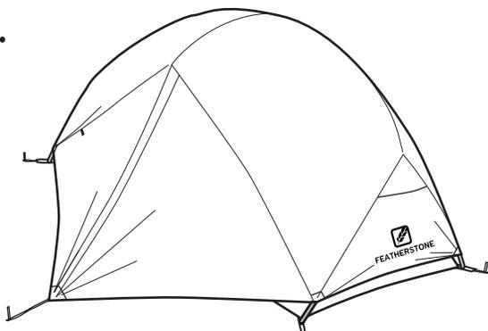
Spread the rainfly over the tent. Buckle down the corners, and tightly fasten each corner when buckled. Stretch the vestibule until it is fully taut and stake it down (do this for the other side as well).
