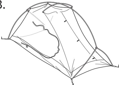
Insert pole-tips into the grommets for both sides. Once fastened, insert the ridge pole-tips found in the middle of the tent.
