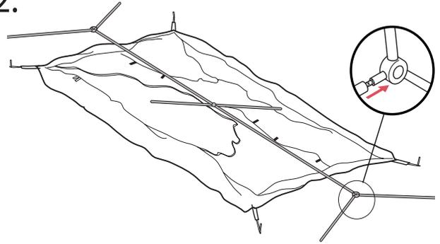
Lay the tent body on an even ground or footprint and stake the four corners of the tent body. Set the poles making sure all pole sections are aligned with the corresponding grommets.
