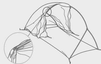
For a quick and ultra light setup, skip steps 2-4. Attach tent poles onto the grommets of the footprint and spread rainfly over the tent. Stretch the vestibule until it is fully taut and stake down (see Step 5).
