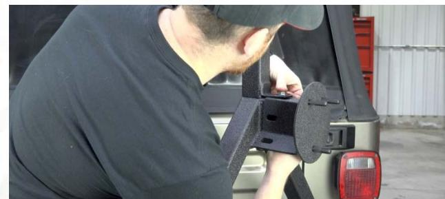
Install the 12mm bolt, with washers and nyloc nut, through the back of the tire carrier and brake light bar.
