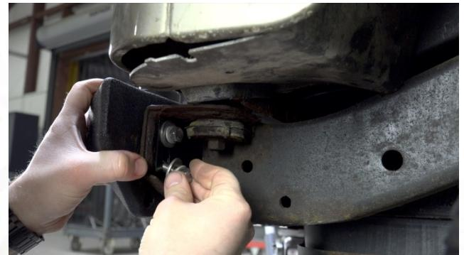
Insert a flat washer, lock washer, and 10mm bolt through the backing plate and into the rear bumper. **Do not fully tighten at this time.** You will need some room to move the bumper around as you install the other bolts. Repeat for all locations.
