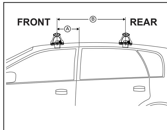
\* Open doors. Pull rubber door seal back. Fit clamp.
