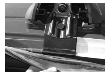
\* After cross bars and clamp are correctly fitted re-fit the rubber door seal.
