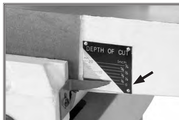
Figure 52. Depth scale adjusted to "0" position.
