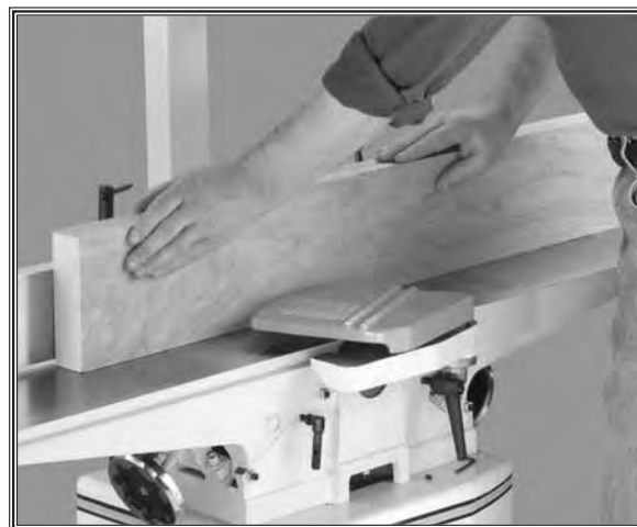
Figure 32. Typical edge jointing operation.
