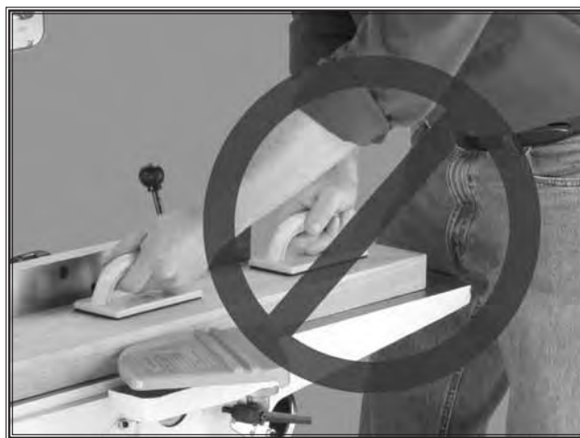
Figure 5. Never stand directly behind the workpiece!
