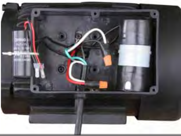
Motor Junction Box
