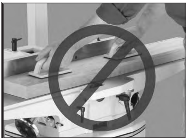
Figure 4. Never plane/edge-joint with the guard removed!
