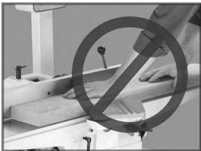
Figure 3. Never surface plane without push blocks!
