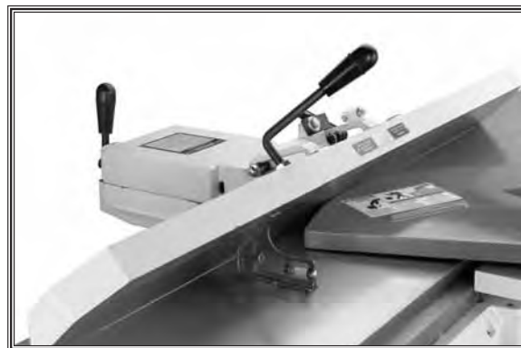
Figure 53. Fence adjusted 45° inward.
