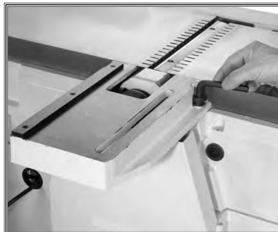
Figure 12. Installing fence bracket.
