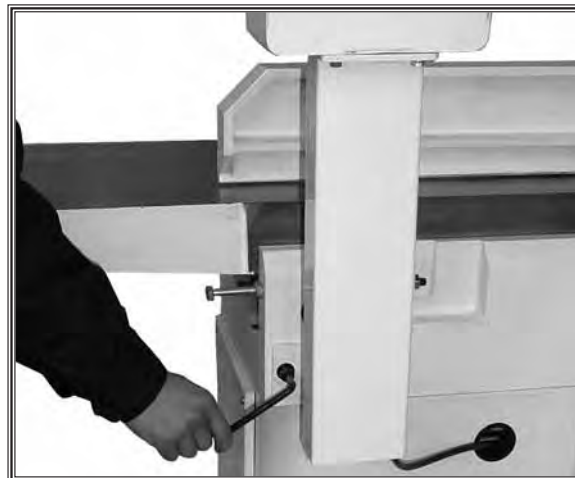
Figure 16. Mounting pedestal in upright position.
