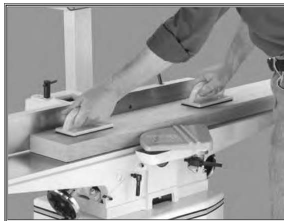
Figure 30. Typical surface planing operation.
