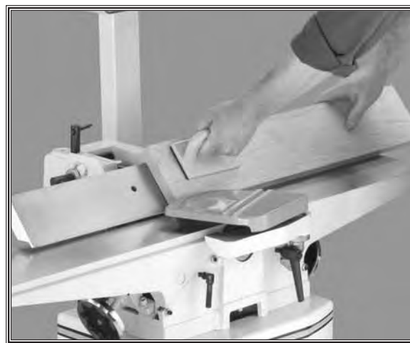
Figure 34. Typical bevel cutting operation.
