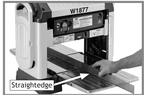
Figure 17. Aligning extension tables.
